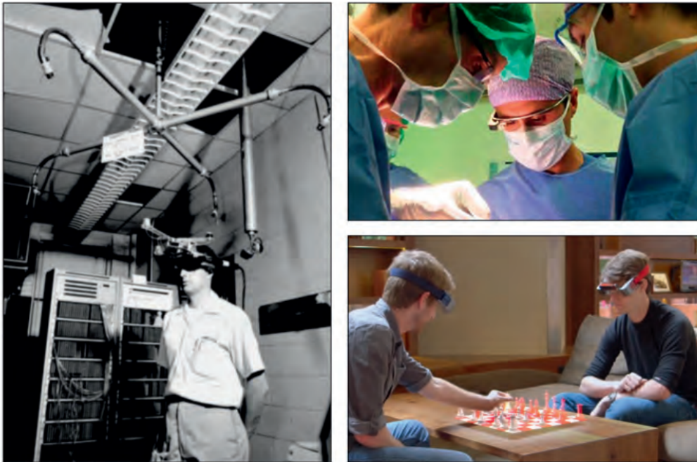
Figure 6: Examples of head mounted AR displays that allow users to visualize virtual content in a real environment. Left: the set-up of Ivan Sutherland developed in 1968, where the display was attached to the ceiling ( https://lookingglassxr.com/augmented-reality ). Top right: Google Glass used in 2013 during orthognathic surgery in the Radboudumc. Lower right: the Meta Glasses allowed users to interact with virtual chess pieces in a real world setting ( https://www.cnet.com/science/meta ).
