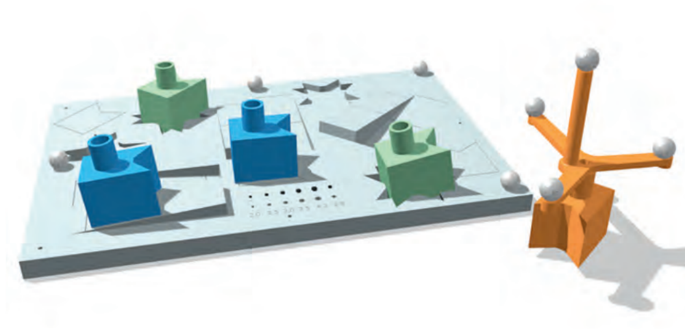
Figure 2: The virtual design of the measuring board and V-shaped tracked cube (orange). The cube was virtually aligned with specific locations on the measuring board. In this figure, the cubes are shown at tight-fitting positions (green) and loose-fitting positions (blue).
