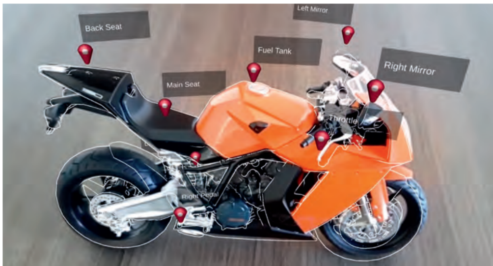
Figure 12: Example of AI object tracking. A deep neural network is used to match the virtual model of a motorcycle (white lines), including the tags, on a real physical object of a motorcycle ( https://www.ptc.com/en/products/vuforia ).
